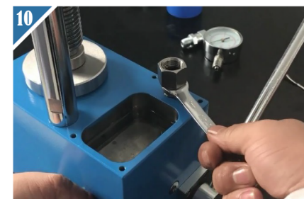
10 Install digital meter special pressure gauge connection column.
