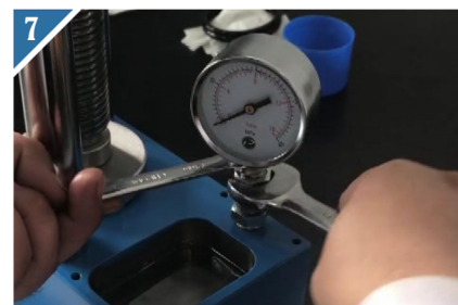
7 Separate the pressure gauge from the pressure gauge column.
