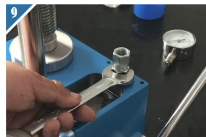
9 Remove the pressure gauge connection post .
